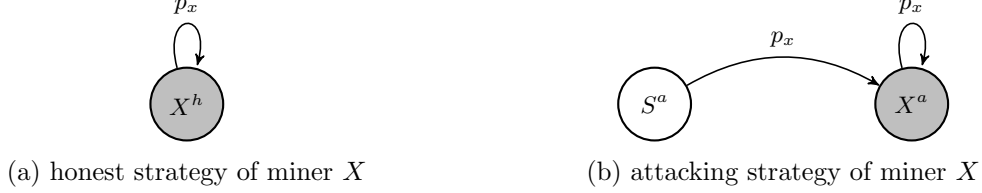
Figure 2: The honest strategy (cf. Figure 2a) and the deviation from the honest strategy (cf. Figure 2b) modeled with discrete Markov chains. All states with a nonzero payout for miner X are highlighted in gray. We transition between states with every block. Note that for all remaining probabilities, the Markov process enters an absorbing state and X 's consecutive turns as a proposer finish.
